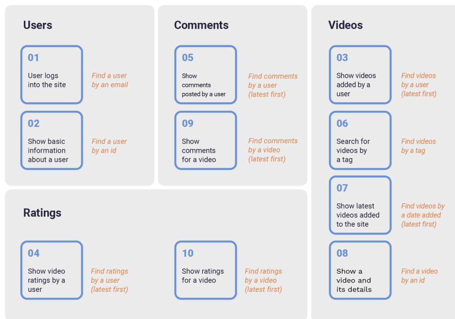
FIGURE 5 Identifying the queries required to support the application workflow
